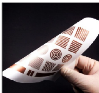
紙基板上への印刷 Pattern on a paper substrate Line 1~3 mm, 30 μm thickness
